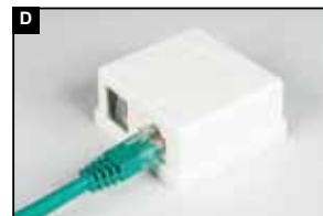
Snap the plug in place.
