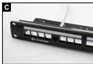
Insert the jack into the mounting location properly.
