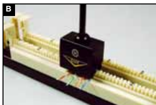
Terminate wires using Linkbasic tool (P/N: TLB01) or equivalent.
