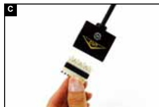
4-pair impact tool seats connecting blocks.
